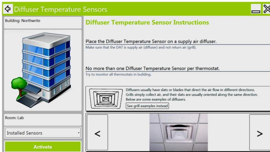
**Figure 2.** A sensor configuration screen from the tablet computer enabling configuration of a diffuser air temperature sensor.
