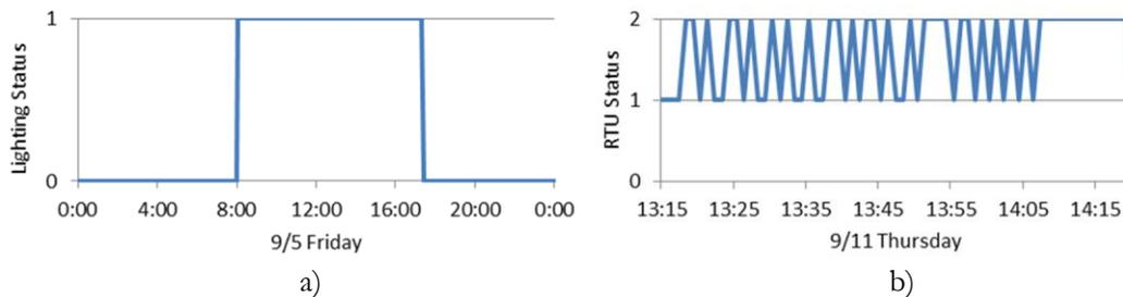
**Figure 5.** Trends from sensors: (a) Site B, trend from a lighting status sensor (1=lighting on, 0=lighting off) on a weekday during the monitoring period, (b) Site B, example trend from a rooftop unit status sensor (0=off, 1= supply fan only on, and 2= compressors, condenser fans, and supply fan all on) during the monitoring period
